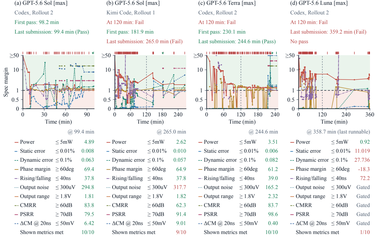
Figure 5 Four six-hour trajectories on one sampling-feedback OTA (task No. 33): early pass (a), pass-then-regress (b), delayed pass (c), and no pass (d). Curves show normalized margins for ten metrics drawn from the verifier’s 15 scoring gates (higher is better); tables report the last runnable circuit, with blocked metrics marked Gated.
